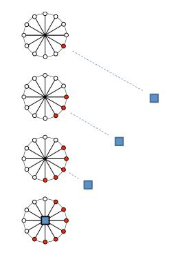
*Figure 6.* The approaching cruiser analogy: as the square object approaches, the patch of active actuators expands
