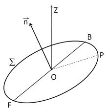
Figure 7. Vertical axis OZ associated with the artificial horizon provided by an aircraft's navigation instrument, and the vertical perceived by the pilot (vector  $\vec{n}$ ) associated with the plane of the device,  $\sum$
