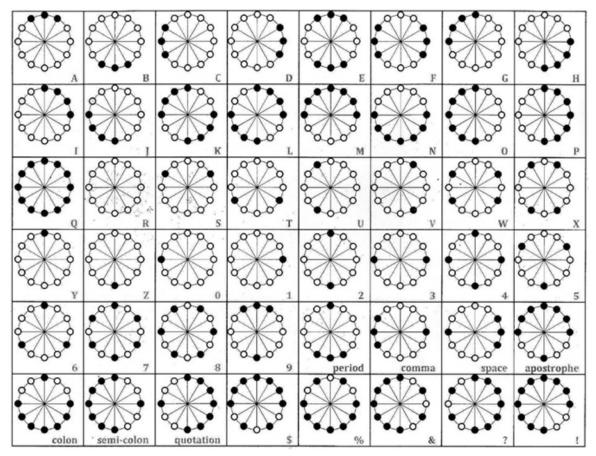
Table 4: Example of a tactile alphabet based on the tactile patterns generated by 12 actuators
